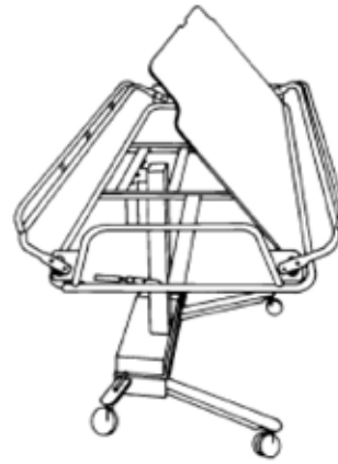
Figure 18 - Cleaning Shower Trolley
