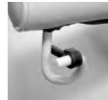
6. Check mounting bolts of actuator top and bottom. Pay particular attention to top bolt hole for elongation.
