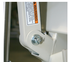
ARM TO MAST
