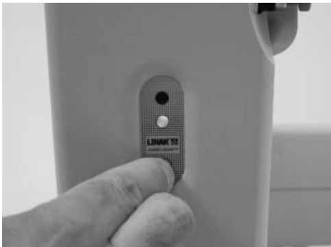
Figure 28 - Hold for electric emergency down
