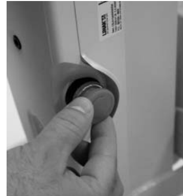
Figure 11 - Emergency Stop button
