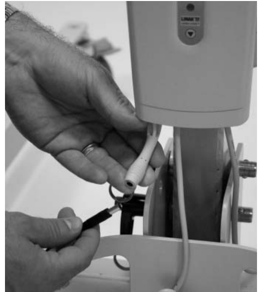
Figure 27 - Charging the EZ Light Lift
